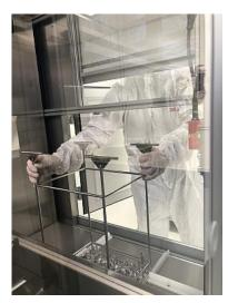
After final cleaning, the parts are discharged into the cleanroom. Consistent monitoring and the comparison of process parameters with validated values ensure that 'bad baskets' are eliminated before they reach the cleanroom.
