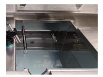
Thanks to the newly developed Acoustic Performance Measurement (APM) system, the ultrasound frequency and output can be monitored and documented in-line at each processing station for each batch.
