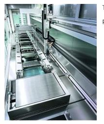
The modular final cleaning system has seven wet stations for cleaning, passivation, neutralization, and rinsing, as well as a vacuum dryer.
