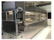
The system concept, which is based on standardized modules, enables the ultrasonic immersion cleaning systems to be individually configured for intermediate and final cleaning applications - also with direct connection to a cleanroom.
