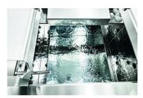
The standard two-sided overflow creates an uninterrupted flow that enhances the intensive treatment of the parts. It also guarantees that cleaned-off contaminants are immediately discharged from the treatment tanks.
