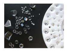
To prevent the coated precision optics from becoming damaged during the cleaning process, in which they are rotated at speeds of up to 1,500 rpm, they are placed in special holders.
