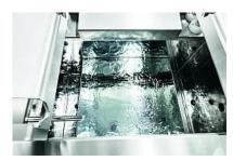
The standard two-sided overflow creates an uninterrupted flow that enhances the intensive treatment of the parts. It also ensures that cleaned-off contaminants are immediately removed from the baths.
