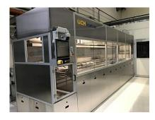
The machine, which is based on standardized modules for washing, rinsing, and drying, not only meets exceptional cleanliness requirements for final cleaning but is also extremely cost-efficient.
