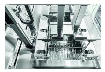
The standard integrated transport system with servo drive means that a lift-out device can be installed for pre-drying the parts after the last rinse cycle if desired.
