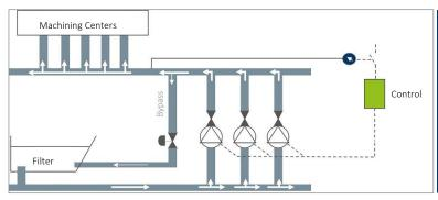
Because the constant pressure control typically implemented in filtration systems for cooling lubricants and other supply systems provide only coarse pressure control, an excessive amount of unused medium has to be fed back to the filtration system via a bypass line. The energy required for this is wasted.
