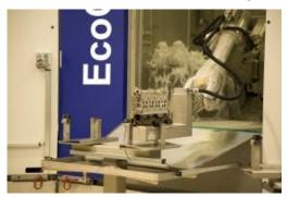
Energy efficiency measures yielded an approx. 30 percent reduction in the electric power and water consumption of an EcoCFlex Classic robot cell that had been in service for several years.
